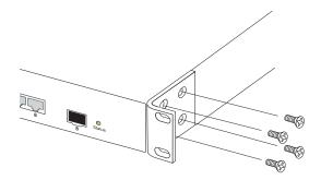
Figure 3-2 Attaching the Brackets
